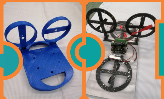
A prototype of a hovercraft made by 3D printing
